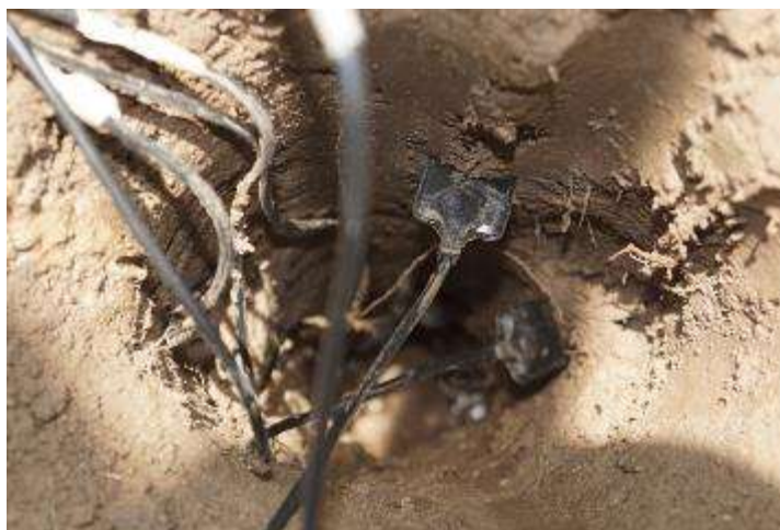
Installation of soil moisture monitoring sensors
