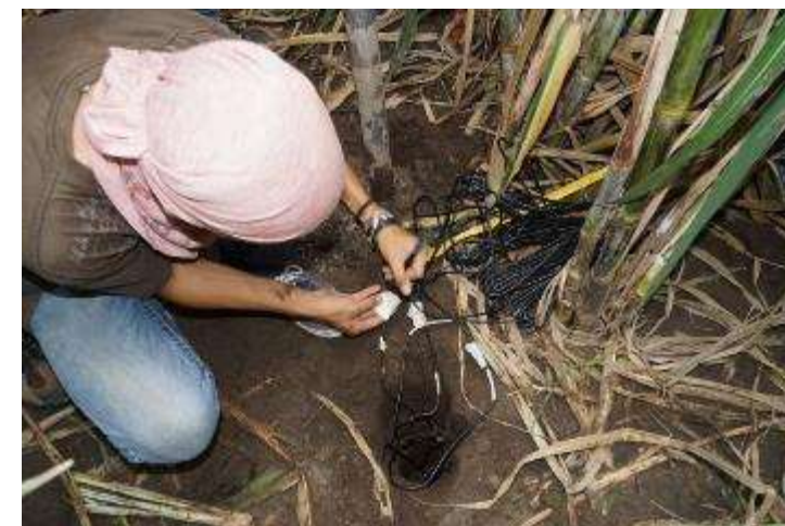
Installation of soil moisture monitoring sensors
